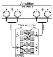
When using the double (A + B) sets of speakers, make sure that you select the "A + B" position with your amplifier.
